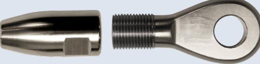
Apply Loctite 262 on threads and lightly screw the two parts together. Unscrew and check both threads are filled with Loctite.
