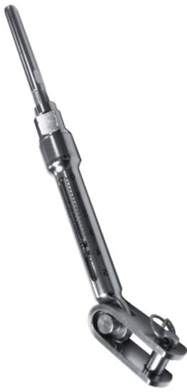
A highly sophisticated rigging screw from the Blue Wave racing line. It features an adjustment nut in black chromed high quality alu bronze, engraved calibration scale for fast and accurate adjustment of the rig tension and an extra long thread terminal.
