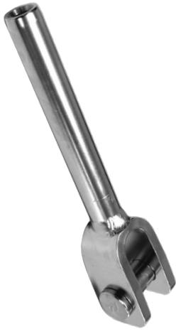
The wide range of hand welded fork terminals by Blue Wave has been setting standards for many years. Featured here are the most common size/fork variations - all with wire size and swage depth marking. Fork terminals are among the most commonly used wire end fittings. They are normally attached to pre-drilled anchor plates or steel constructions. Also used in combination with toggles, eyes or U-bolts.
