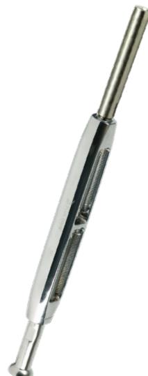
Body chromed according to DS/EN ISO 1456 class 4 with one layer of nickel thickness minimum 0,025 mm and one layer of chrome thickness minimum 0,003 mm. Bright finish.
