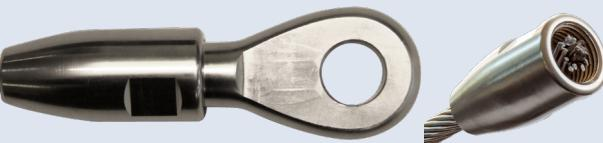
As a precaution take the terminal apart and visually check that the strands lay evenly around the cone and fit into the wire former (top part). Finally re-assemble as above and allow the Loctite to dry.
