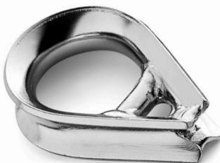
The reinforced thimble is based on the standard thimble but extra force is attained by the addition of a welded bar and ends being welded together. A good choice for wire and UHMWPE ropes.
