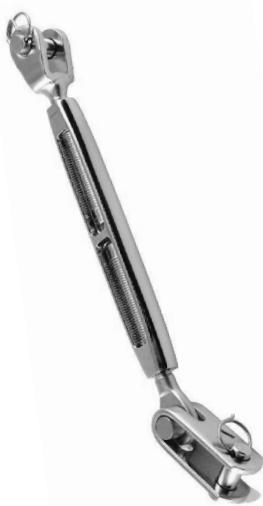
Body chromed according to DS/EN ISO 1456 class 4 with one layer of nickel thickness minimum 0,025 mm and one layer of chrome thickness minimum 0,003 mm. Bright finish.
